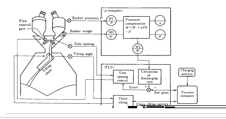
Fig. 15 Charging rate control system
