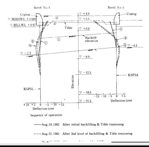
Fig. 11 Deflection of sheet piles of sheet pile double wall structure
