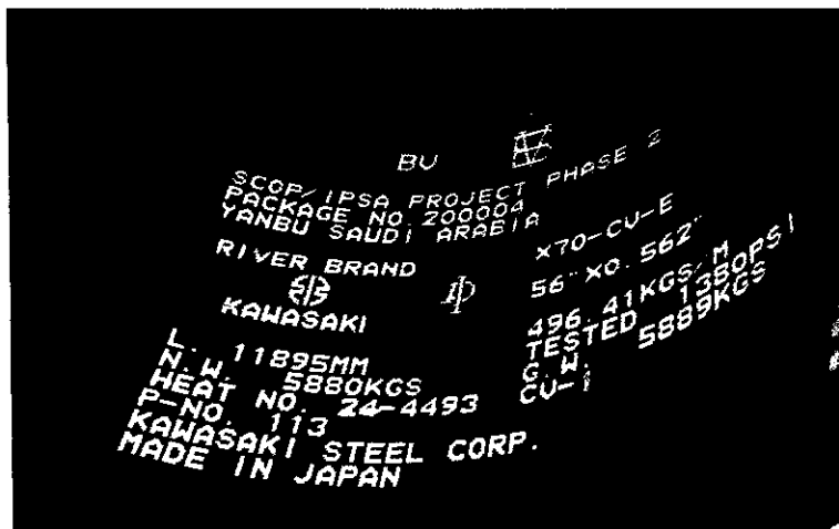
Photo 2 Marking on the inside surface
